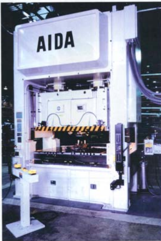
Above: The NSU's massive one-piece frame, the rigidity of the press and its low clearance minimises elongation during parts production for improved accuracy
