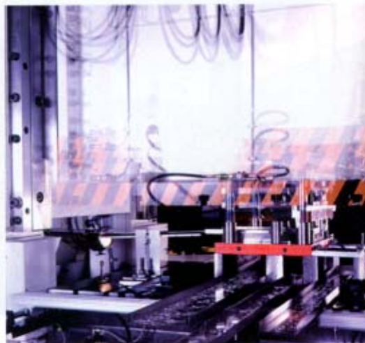
Above: The NSU's massive one-piece frame, the rigidity of the press and its low clearance minimises elongation during parts production for improved accuracy
